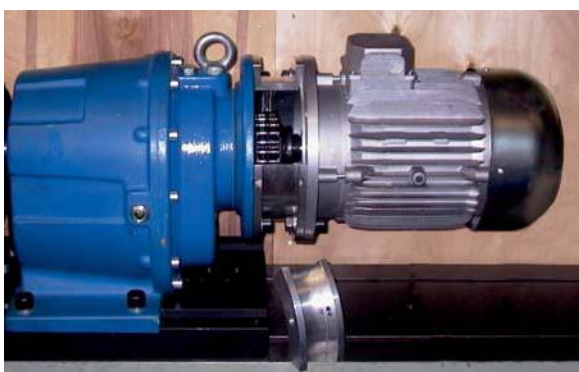
Spacer type A with inspection for check and torque limiter calibration.
